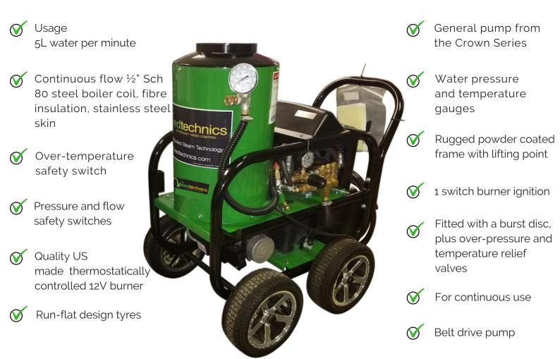
Note: The unit has a built-in hose reel connection; It can be priced with or without a manual wind hose reel to wind up your hose. It also comes with a 10m extension power cord.
