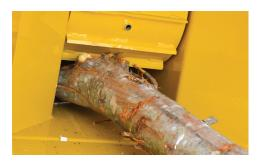
**LARGE RECTANGULAR FEED OPENING.** The large 9"x14" feed opening helps boost productivity by reducing the need to trim heavily branched material before feeding it into the chipper.
