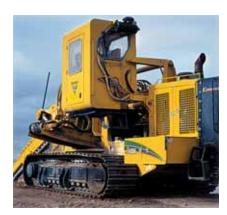
A 600 hp (447 kW) Caterpillar Tier 3 engine delivers the power needed to triumph over tough rock-trenching projects.
