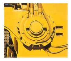
**Dual Rotary Power headshaft motors and a splined headshaft** produce lower speed and higher torque, giving you superior rock penetration and low chain wear for
