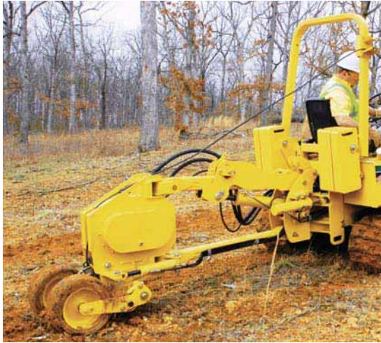
Plow. This attachment installs product up to 24 inches (64 cm) in depth.
