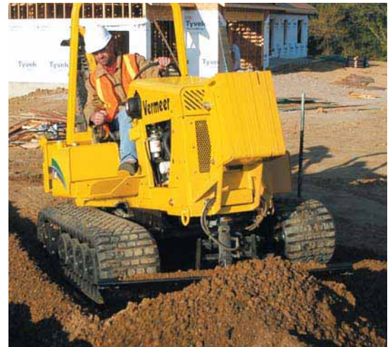
Backfill blade. The blade features a 64-inch extension (163 cm) width with a 30 degree swing angle and a tilt angle of 12 degrees.
