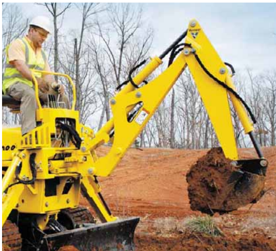
Backhoe. The backhoe features a maximum digging depth of 76 inches (193 cm) with a swing arc of 170 degrees.
