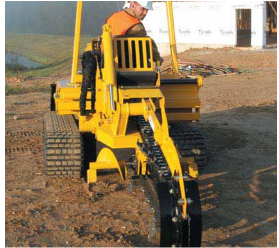
Sliding offset flex trencher. The sliding offset flex trencher offers a maximum digging depth of 60 inches (152 cm) and width of 12 inches (30 cm).
